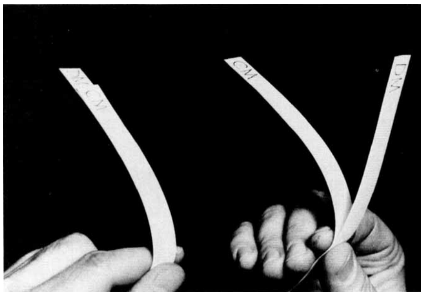
FIG. 2. Test to reveal machine direction (DM) in paper sheet. Strips cut from each of two perpendicular directions are held together horizontally. The stiffer strip is designated DM and the other CM (cross-machine).
